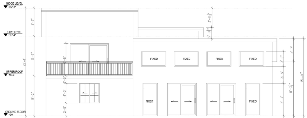
1 FRONT ELEVATION Scale 1"=1/8"
