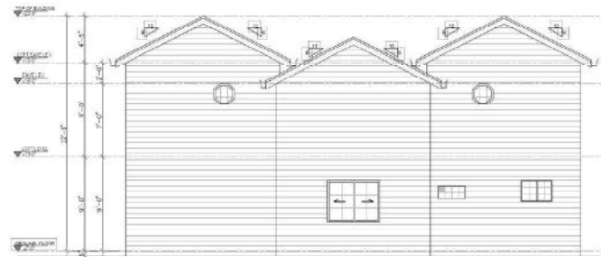
REAR ELEVATION Scale 1/8"=1'
